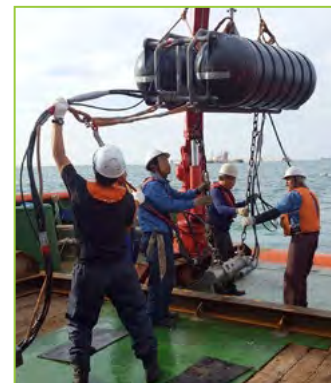
Acoustic energy sources (compressed air) being deployed for ultra-high-resolution 3D seismic data acquisition at the Tomakomai CO 2 storage demonstration project offshore Tomakomai, Hokkaido, Japan.
