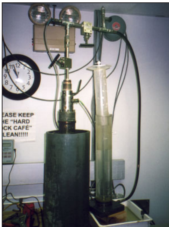
The photo shows the graduated cylinder filling with gas as the ODP Pressure Core Sampler undergoes controlled degassing in the lab aboard the R/V JOIDES Resolution. A maximum of 27.6 gallons (97 liters) of methane from gas hydrates was recovered during Leg 204, a record for this tool.
