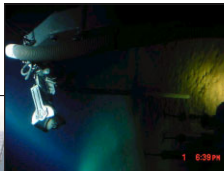
This thermister probe was found to be in good condition with more than three years of thermal recordings. A thermal record captures loop current transit as corroborated by satellite imagery. The event coincided with an increase/decrease of gas vent bubble stream activity in the vicinity of the hydrate mound.
