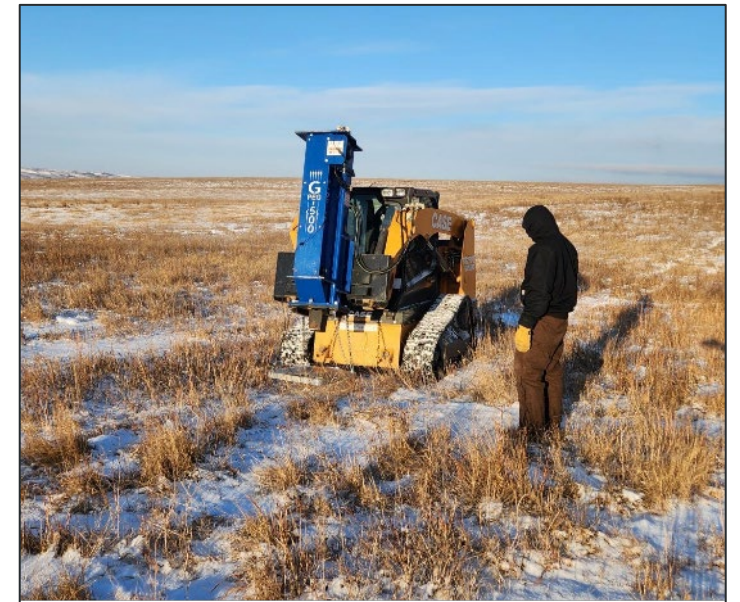
Below: Skid-Steer-Mounted Accelerated Weight Drop (AWD)
